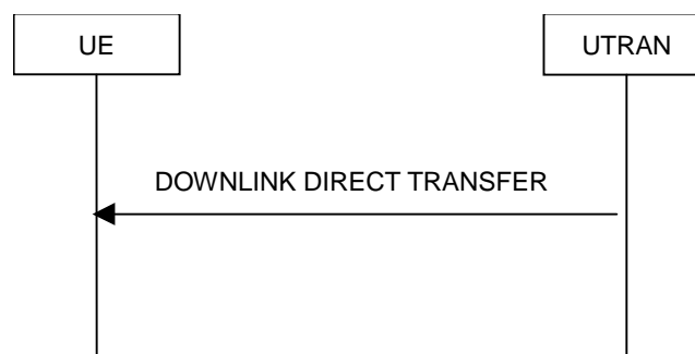
Figure 8.1.9-1: Downlink Direct transfer, normal flow
