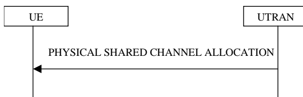
Figure 8.2.7-1: Physical Shared Channel Allocation
