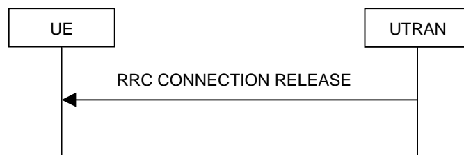
Figure 8.1.4-2: RRC Connection Release procedure on the CCCH
