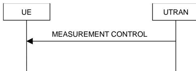
Figure 8.4.1-1: Measurement Control, normal case
