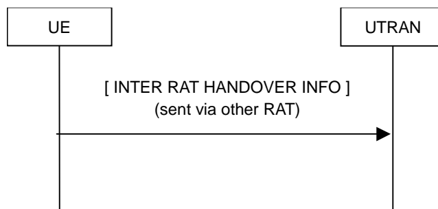
Figure 8.1.16-1: Inter RAT handover information transfer, normal flow
