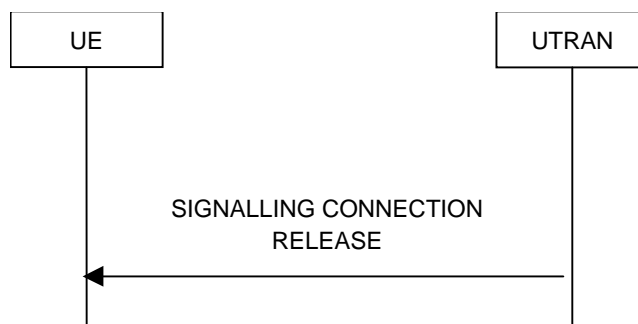
Figure 8.1.13-1: Signalling connection release procedure, normal case
