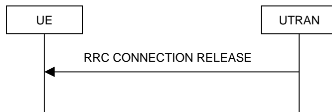
Figure 8.1.4-2: RRC Connection Release procedure on the CCCH
