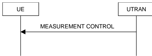
Figure 8.4.1-1: Measurement Control, normal case
