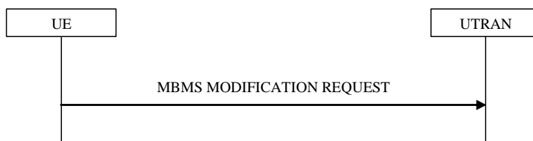
Figure 8.7.6-1: MBMS modification request, normal
