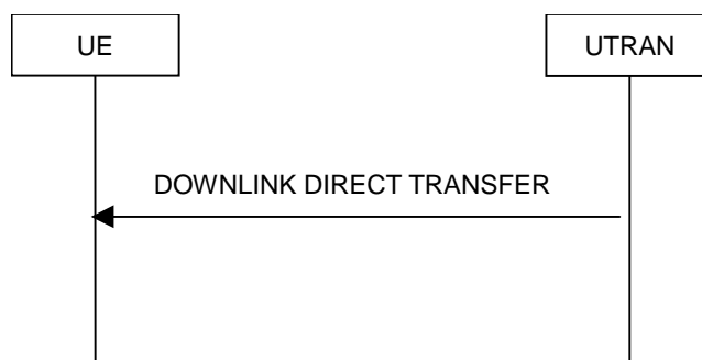
Figure 8.1.9-1: Downlink Direct transfer, normal flow
