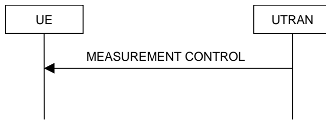
Figure 8.4.1-1: Measurement Control, normal case
