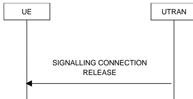
Figure 8.1.13-1: Signalling connection release procedure, normal case
