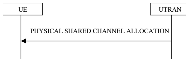
Figure 8.2.7-1: Physical Shared Channel Allocation
