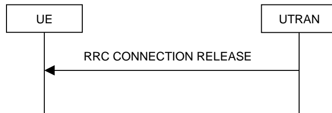
Figure 8.1.4-2: RRC Connection Release procedure on the CCCH
