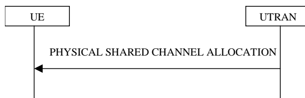
Figure 8.2.7-1: Physical Shared Channel Allocation
