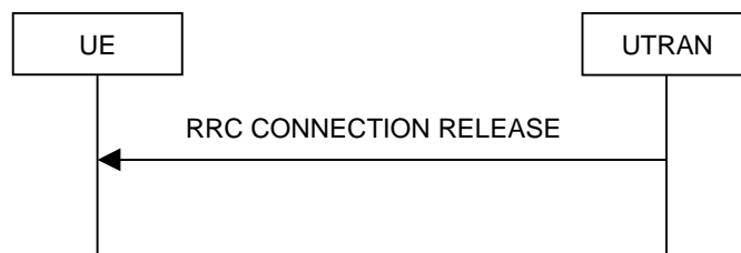
Figure 8.1.4-2: RRC Connection Release procedure on the CCCH
