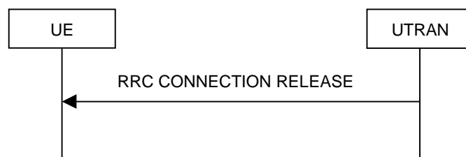
Figure 8.1.4-2: RRC Connection Release procedure on the CCCH
