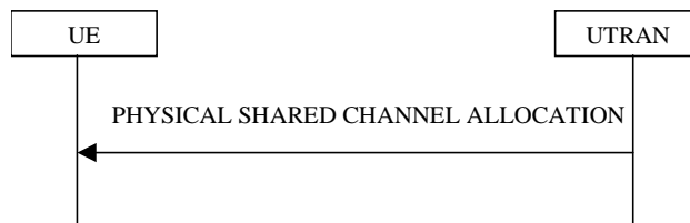
Figure 8.2.7-1: Physical Shared Channel Allocation
