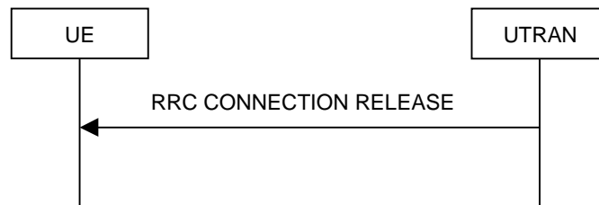
Figure 8.1.4-2: RRC Connection Release procedure on the CCCH
