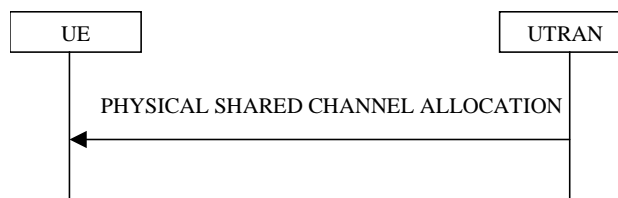
Figure 8.2.7-1: Physical Shared Channel Allocation
