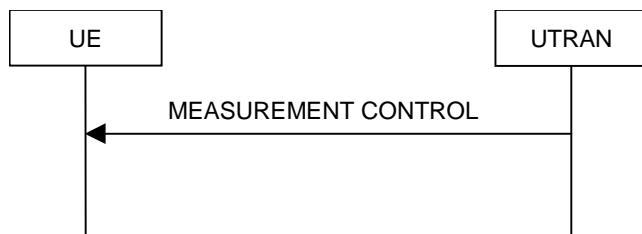
**Figure 8.4.1-1: Measurement Control, normal case**
