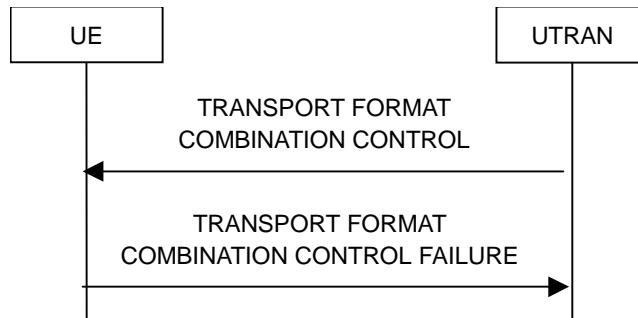
**Figure 8.2.5-2: Transport format combination control, failure case**
