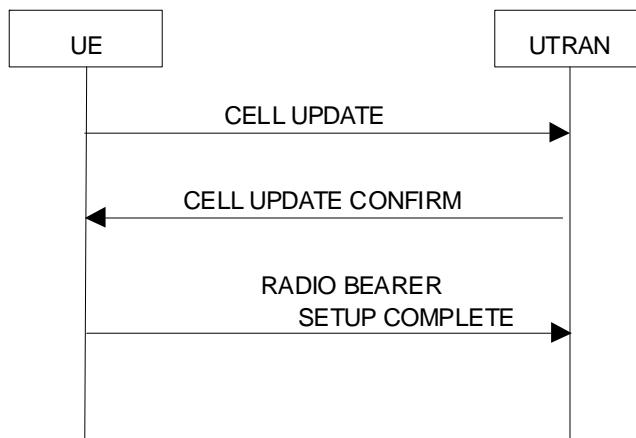
**Figure 8.3.1-6a: Cell update procedure with radio bearer setup**
