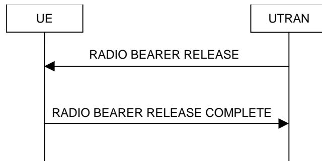
**Figure 8.2.2-5: Radio Bearer Release, normal case**
