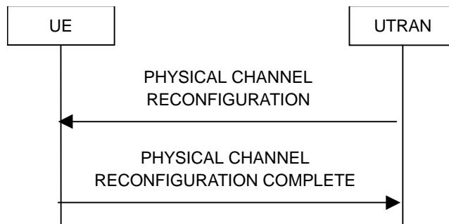
**Figure 8.2.2-9: Physical channel reconfiguration, normal flow**
