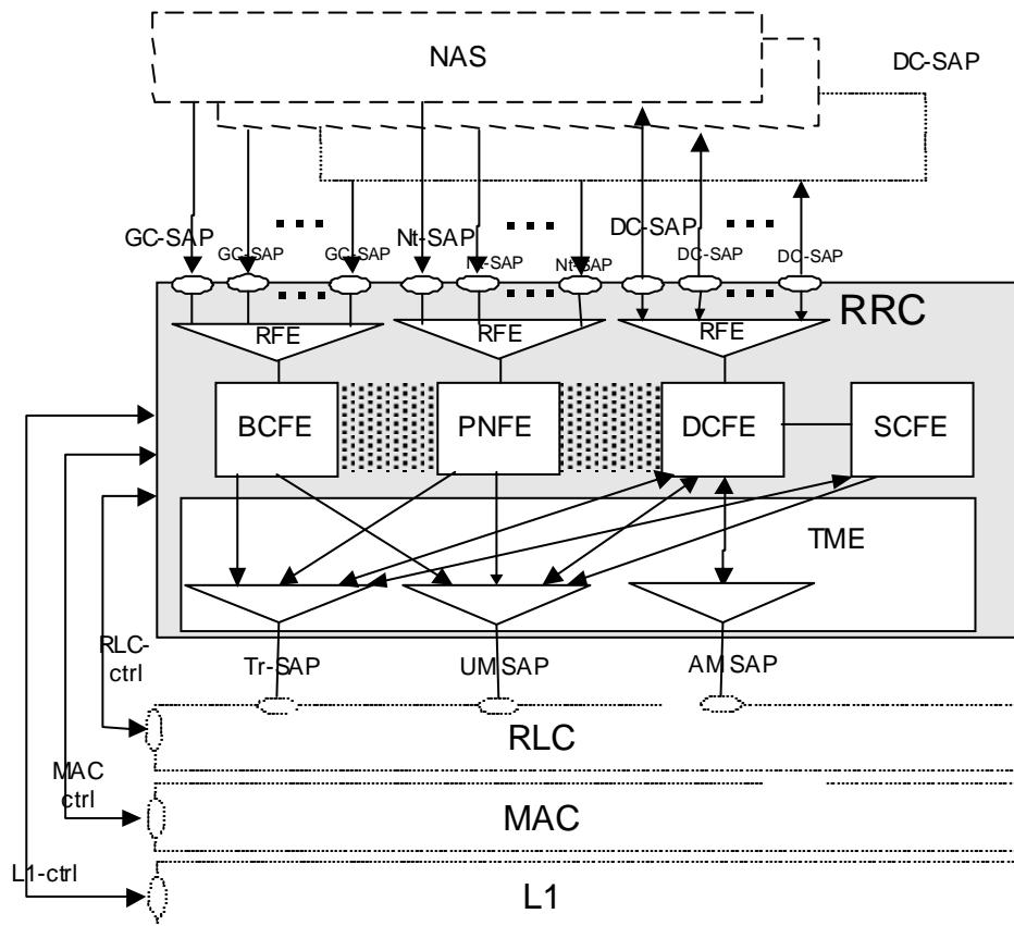
Figure 4.2-3: UTRAN side RRC model (DS-41 System)
