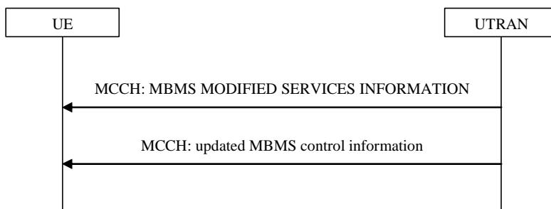
**Figure 8.7.3-1: MBMS notification on MCCH**
