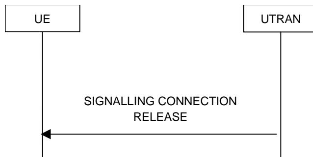
**Figure 8.1.13-1: Signalling connection release procedure, normal case**
