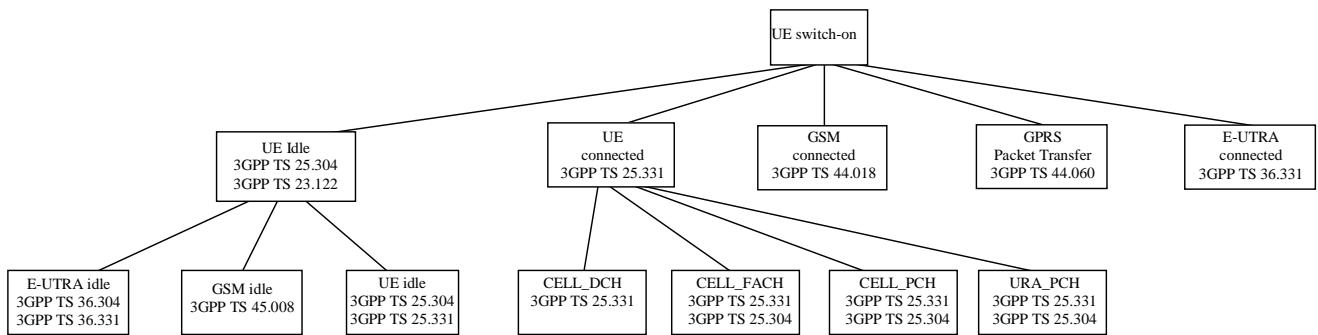
**Figure 4.1-1: Mapping of UE state to 3GPP Specifications**
