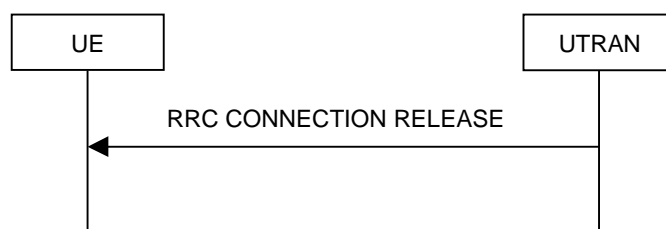
Figure 8.1.4-2: RRC Connection Release procedure on the CCCH
