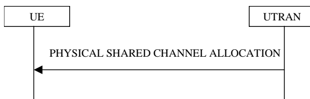
Figure 8.2.7-1: Physical Shared Channel Allocation
