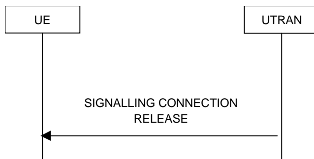
Figure 8.1.13-1: Signalling connection release procedure, normal case
