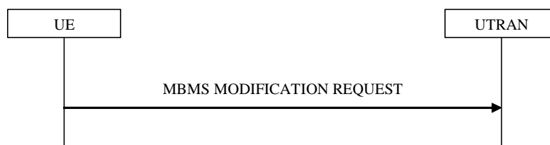
Figure 8.7.6-1: MBMS modification request, normal
