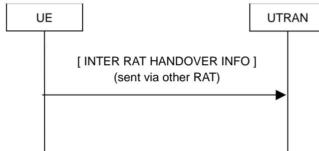
Figure 8.1.16-1: Inter RAT handover information transfer, normal flow
