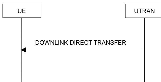
Figure 8.1.9-1: Downlink Direct transfer, normal flow
