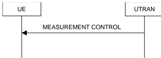
Figure 8.4.1-1: Measurement Control, normal case
