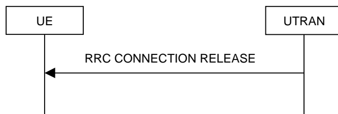
Figure 8.1.4-2: RRC Connection Release procedure on the CCCH
