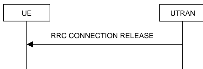
Figure 8.1.4-2: RRC Connection Release procedure on the CCCH
