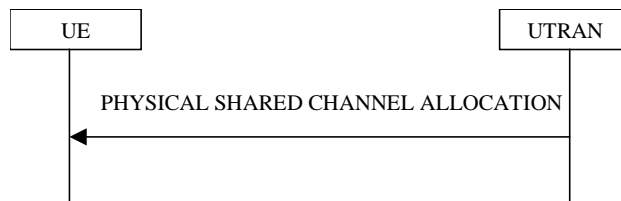
Figure 8.2.7-1: Physical Shared Channel Allocation
