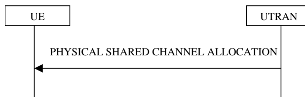
Figure 8.2.7-1: Physical Shared Channel Allocation
