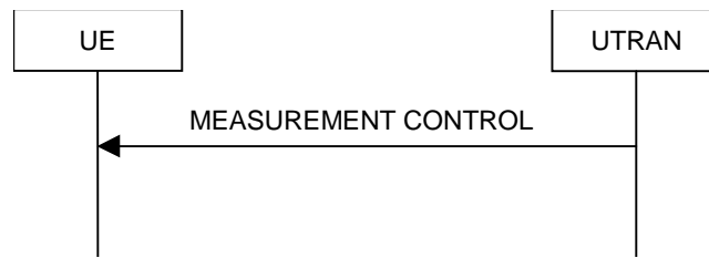
Figure 8.4.1-1: Measurement Control, normal case
