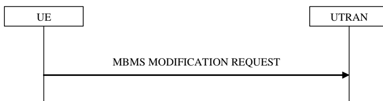
Figure 8.7.6-1: MBMS modification request, normal
