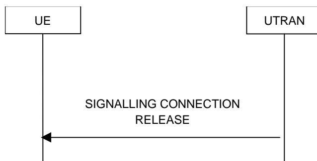
Figure 8.1.13-1: Signalling connection release procedure, normal case
