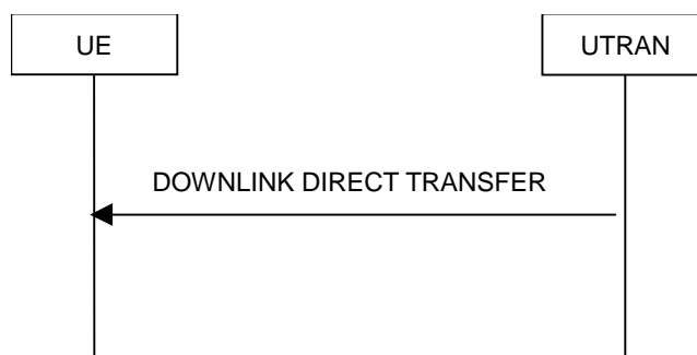
Figure 8.1.9-1: Downlink Direct transfer, normal flow
