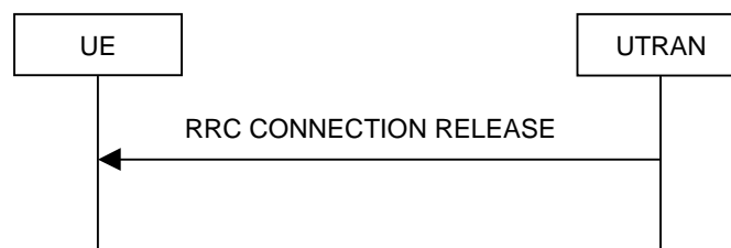
Figure 8.1.4-2: RRC Connection Release procedure on the CCCH
