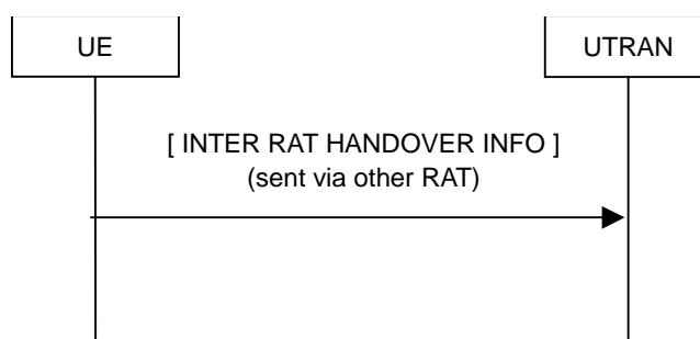
Figure 8.1.16-1: Inter RAT handover information transfer, normal flow
