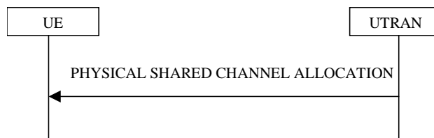
Figure 8.2.7-1: Physical Shared Channel Allocation
