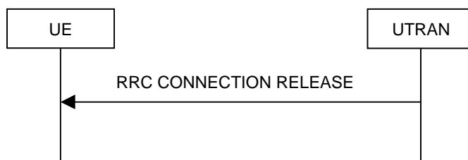
Figure 8.1.4-2: RRC Connection Release procedure on the CCCH
