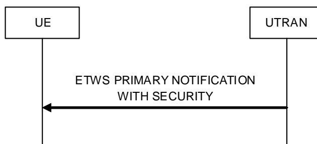
Figure 8.1.17-1: ETWS primary notification with security
