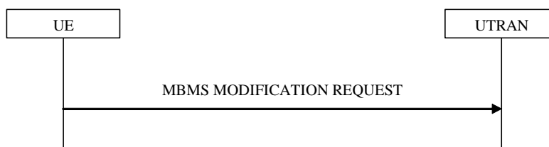
Figure 8.7.6-1: MBMS modification request, normal
