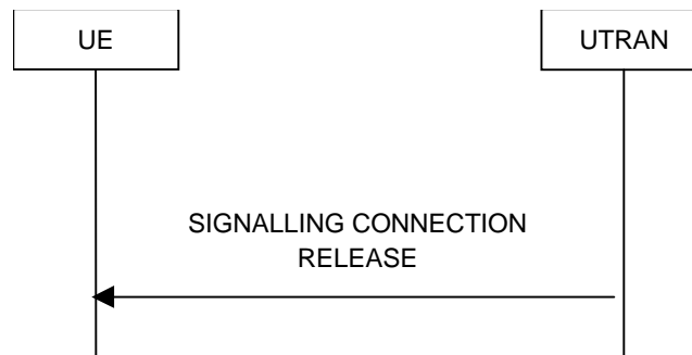
Figure 8.1.13-1: Signalling connection release procedure, normal case
