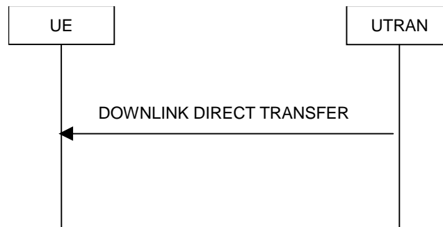
Figure 8.1.9-1: Downlink Direct transfer, normal flow
