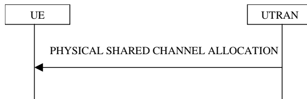
Figure 8.2.7-1: Physical Shared Channel Allocation
