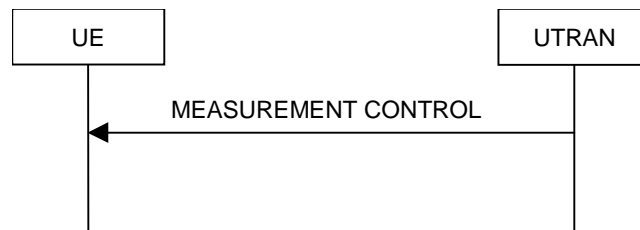
Figure 8.4.1-1: Measurement Control, normal case
