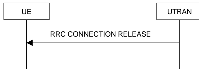
Figure 8.1.4-2: RRC Connection Release procedure on the CCCH
