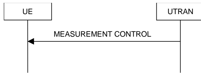
Figure 8.4.1-1: Measurement Control, normal case
