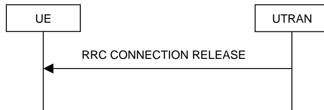
Figure 8.1.4-2: RRC Connection Release procedure on the CCCH
