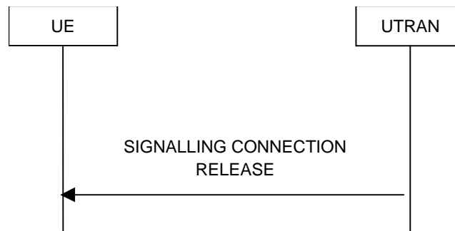
Figure 8.1.13-1: Signalling connection release procedure, normal case
