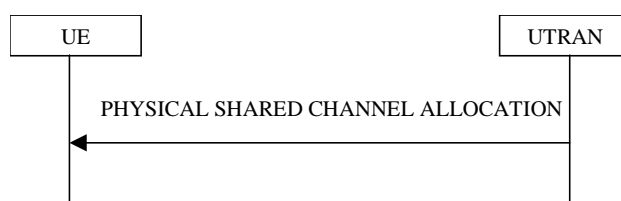
Figure 8.2.7-1: Physical Shared Channel Allocation
