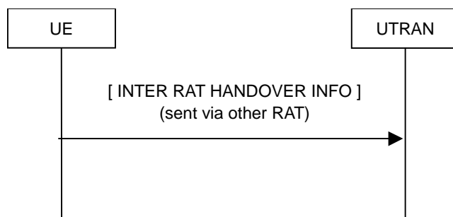
Figure 8.1.16-1: Inter RAT handover information transfer, normal flow
