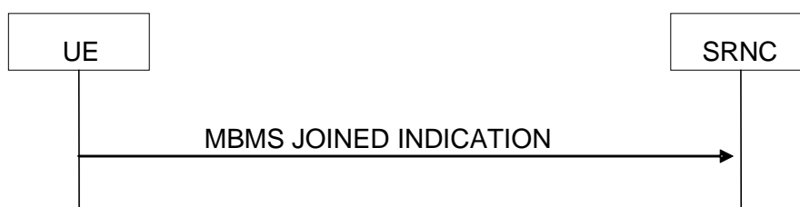
Figure 8.3.6: MBMS joined indication signalling flow
