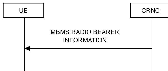
Figure 8.3.3: MBMS radio bearer information signalling flow
