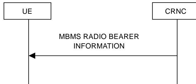
Figure 8.3.3: MBMS radio bearer information signalling flow
