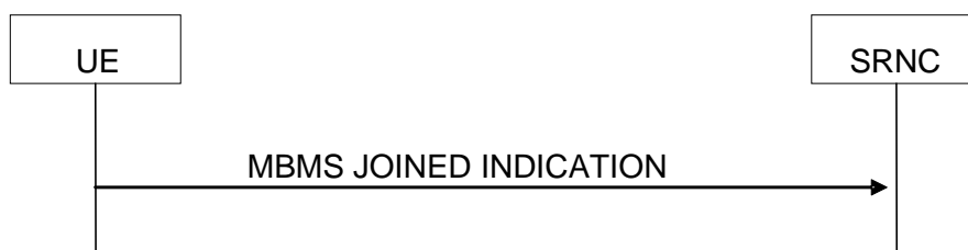
Figure 8.3.6: MBMS joined indication signalling flow
