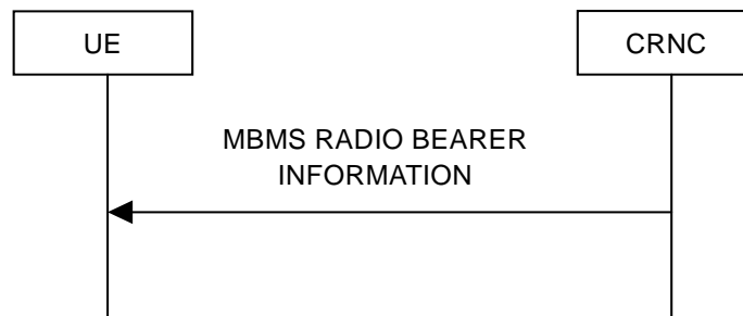
Figure 8.3.3: MBMS radio bearer information signalling flow
