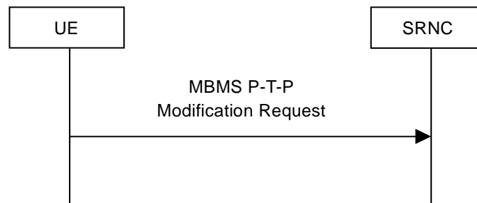
Figure 8.3.9: MBMS P-T-P Modification Request.
