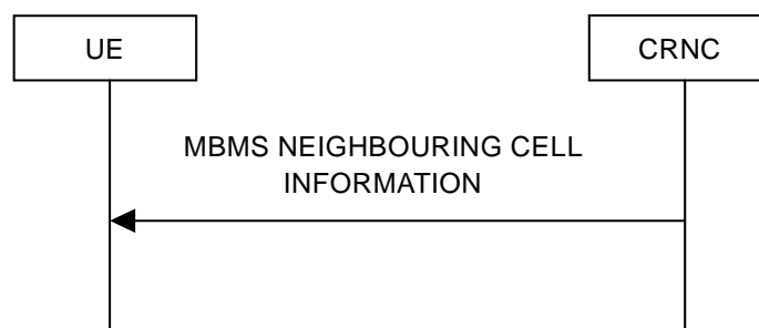
Figure 8.3.5: MBMS Neighbouring Cell Information signalling flow
