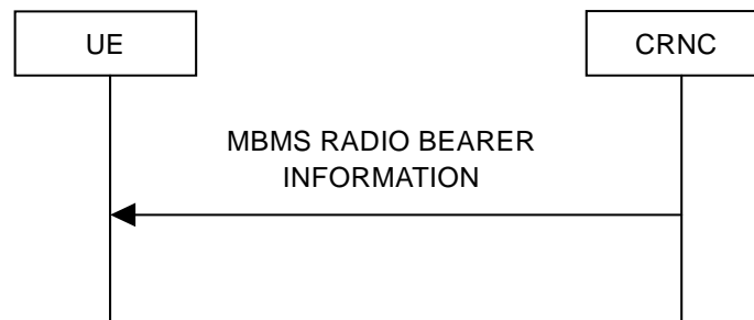
Figure 8.3.3: MBMS radio bearer information signalling flow
