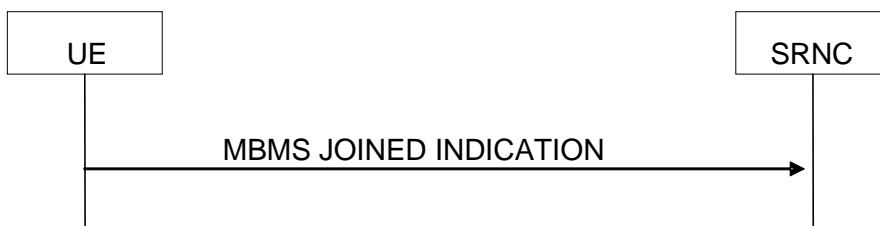
Figure 8.3.6: MBMS joined indication signalling flow
