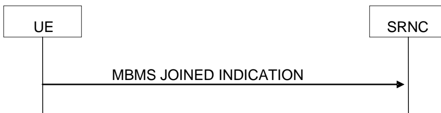
Figure 8.3.6: MBMS joined indication signalling flow
