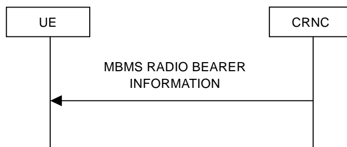
Figure 8.3.3: MBMS radio bearer information signalling flow
