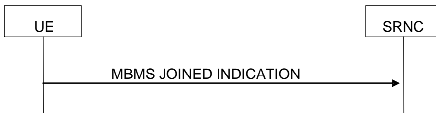
Figure 8.3.6: MBMS joined indication signalling flow
