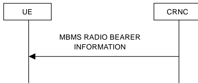
Figure 8.3.3: MBMS radio bearer information signalling flow
