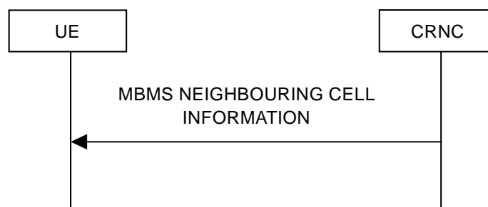
Figure 8.3.5: MBMS Neighbouring Cell Information signalling flow
