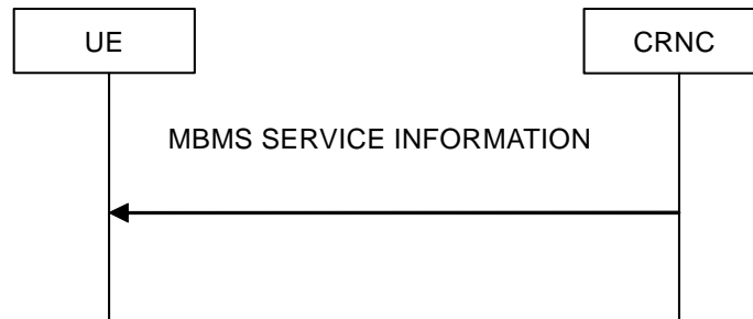
Figure 8.3.2: MBMS service information signalling flow
