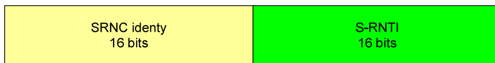
Figure A2.2.1.1: Interpretation of U-RNTI in UE side and RAN side is configured to use the extended RNC ID
