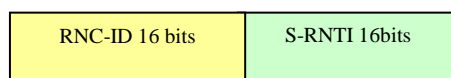
Figure A2.1.1.2: RNC-Side, split of U-RNTI in RNC-ID and S-RNTI in the case of many small RNCs deployed
