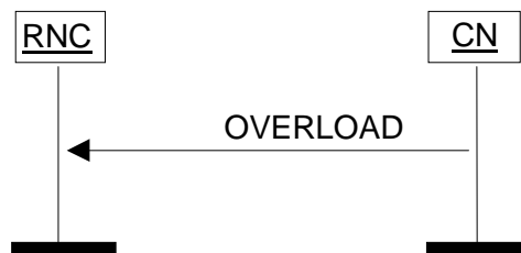
Figure 29: Overload at the CN
