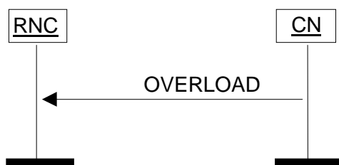
Figure 29: Overload at the CN
