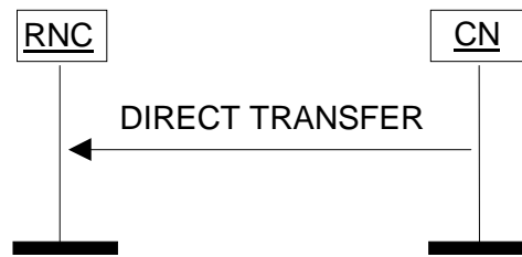
Figure 25: Direct Transfer, CN originated
