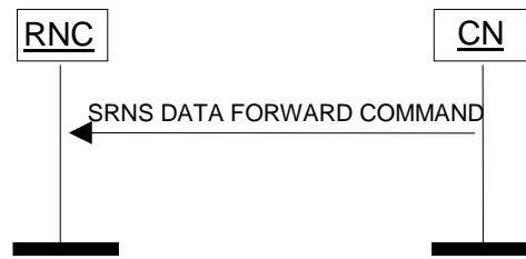
Figure 13: SRNS Data Forwarding Initiation procedure
