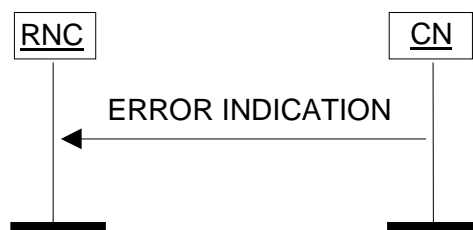
Figure 33: Error Indication procedure, CN originated
