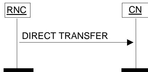
Figure 26: Direct Transfer, RNC originated
