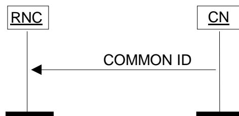
Figure 17: Common ID procedure. Successful operation.
