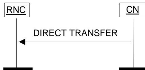
Figure 25: Direct Transfer, CN originated. Successful operation.
