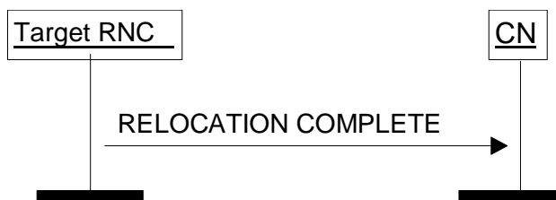
Figure 10: Relocation Complete procedure. Successful operation.
