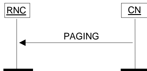
Figure 16: Paging procedure. Successful operation.
