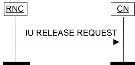
Figure 3: Iu Release Request procedure. Successful operation.
