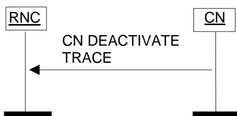
Figure 33: CN Deactivate Trace procedure. Successful operation.
