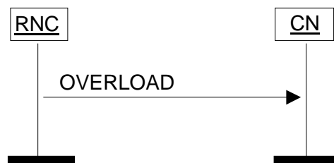
Figure 28: Overload at the UTRAN. Successful operation.
