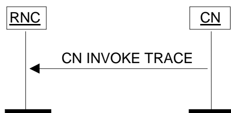
Figure 18: CN Invoke Trace procedure. Successful operation.
