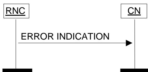
Figure 32: Error Indication procedure, RNC originated. Successful operation.
