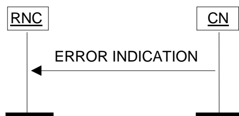
Figure 31: Error Indication procedure, CN originated. Successful operation.
