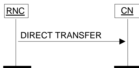
Figure 26: Direct Transfer, RNC originated. Successful operation.
