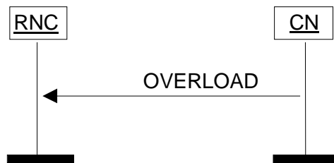
Figure 27: Overload at the CN. Successful operation.
