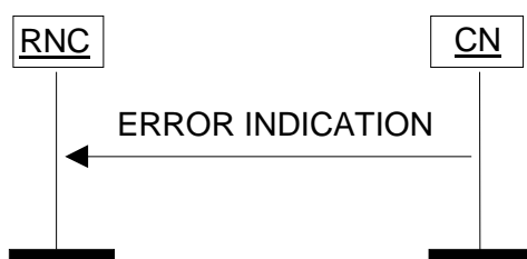
Figure 31: Error Indication procedure, CN originated. Successful operation.
