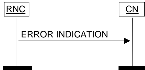
Figure 32: Error Indication procedure, RNC originated. Successful operation.
