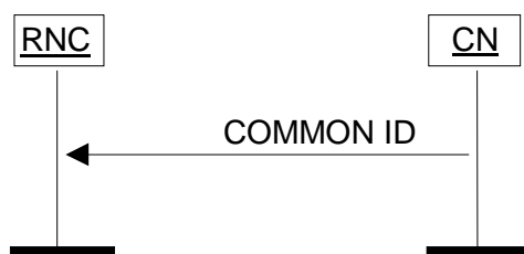
Figure 17: Common ID procedure. Successful operation.
