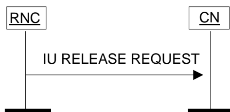
Figure 3: Iu Release Request procedure. Successful operation.
