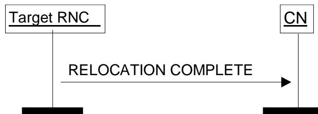
Figure 10: Relocation Complete procedure. Successful operation.
