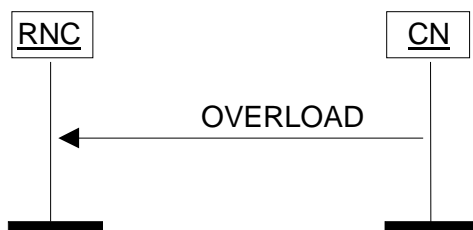
Figure 27: Overload at the CN. Successful operation.
