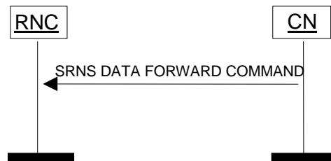
Figure 13: SRNS Data Forwarding Initiation procedure. Successful operation.
