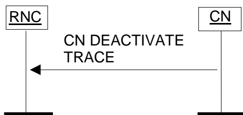
Figure 33: CN Deactivate Trace procedure. Successful operation.
