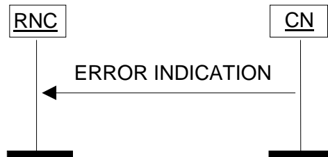
Figure 31: Error Indication procedure, CN originated. Successful operation.
