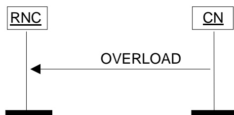
Figure 27: Overload at the CN. Successful operation.
