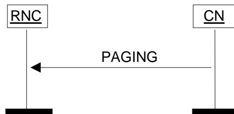
Figure 16: Paging procedure. Successful operation.
