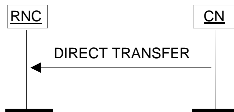
Figure 25: Direct Transfer, CN originated. Successful operation.
