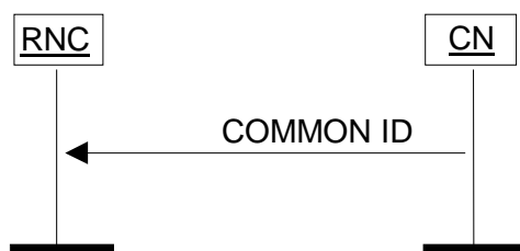
Figure 17: Common ID procedure. Successful operation.
