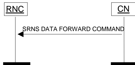
Figure 13: SRNS Data Forwarding Initiation procedure. Successful operation.
