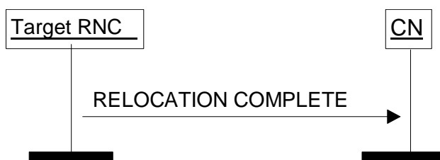
Figure 10: Relocation Complete procedure. Successful operation.
