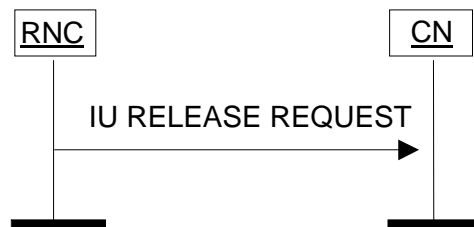
Figure 3: Iu Release Request procedure. Successful operation.
