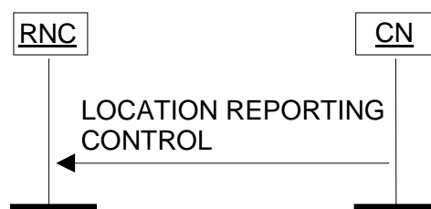
Figure 21: Location Reporting Control procedure. Successful operation.
