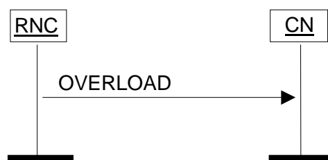
Figure 28: Overload at the UTRAN. Successful operation.
