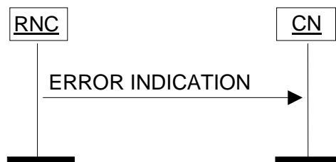
Figure 32: Error Indication procedure, RNC originated. Successful operation.
