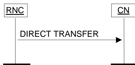
Figure 26: Direct Transfer, RNC originated. Successful operation.
