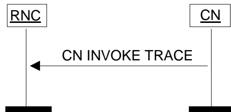
Figure 18: CN Invoke Trace procedure. Successful operation.
