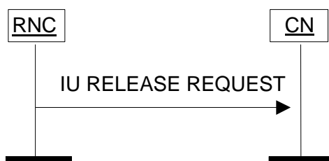
Figure 3: Iu Release Request procedure. Successful operation.
