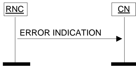
Figure 32: Error Indication procedure, RNC originated. Successful operation.
