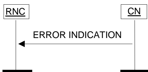
Figure 31: Error Indication procedure, CN originated. Successful operation.
