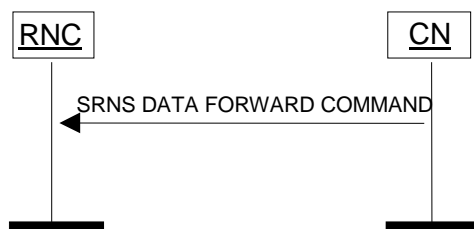
Figure 13: SRNS Data Forwarding Initiation procedure. Successful operation.
