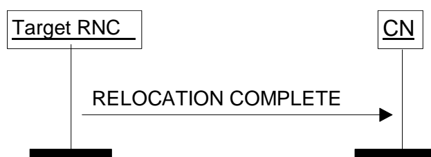
Figure 10: Relocation Complete procedure. Successful operation.
