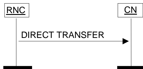
Figure 26: Direct Transfer, RNC originated. Successful operation.
