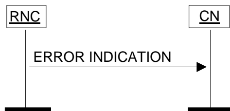
Figure 32: Error Indication procedure, RNC originated. Successful operation.
