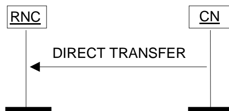
Figure 25: Direct Transfer, CN originated. Successful operation.
