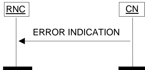
Figure 31: Error Indication procedure, CN originated. Successful operation.
