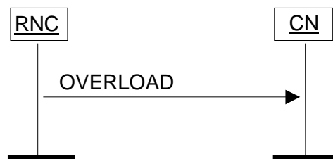
Figure 28: Overload at the UTRAN. Successful operation.
