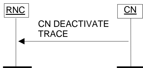
Figure 33: CN Deactivate Trace procedure. Successful operation.
