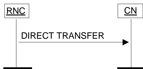
Figure 26: Direct Transfer, RNC originated. Successful operation.
