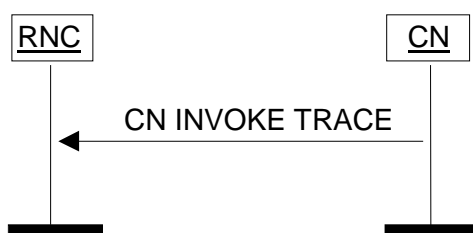
Figure 18: CN Invoke Trace procedure. Successful operation.
