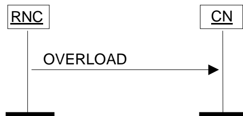
Figure 28: Overload at the UTRAN. Successful operation.
