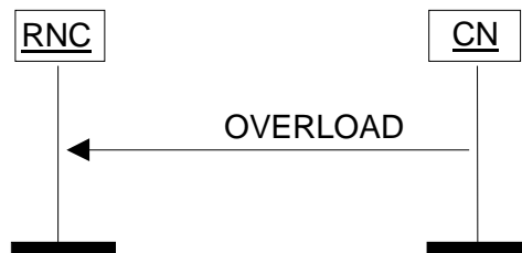
Figure 27: Overload at the CN. Successful operation.
