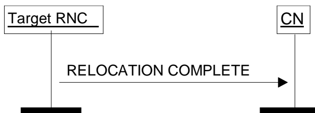
Figure 10: Relocation Complete procedure. Successful operation.
