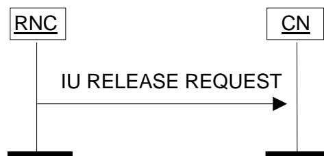
Figure 3: Iu Release Request procedure. Successful operation.
