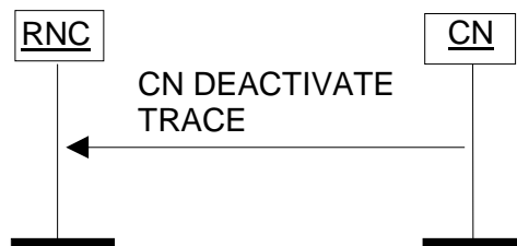
Figure 33: CN Deactivate Trace procedure. Successful operation.
