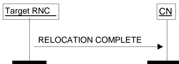
Figure 10: Relocation Complete procedure. Successful operation.
