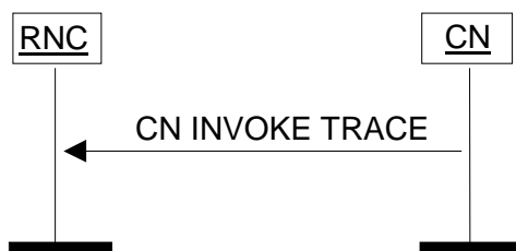
Figure 18: CN Invoke Trace procedure. Successful operation.
