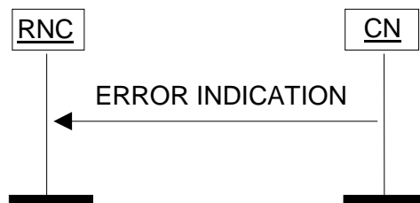
Figure 31: Error Indication procedure, CN originated. Successful operation.
