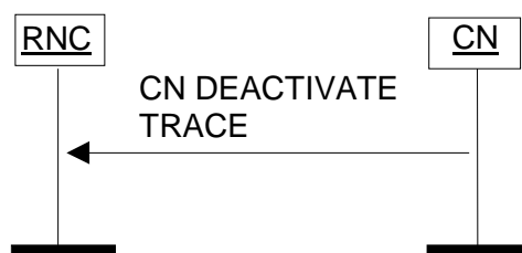
Figure 33: CN Deactivate Trace procedure. Successful operation.
