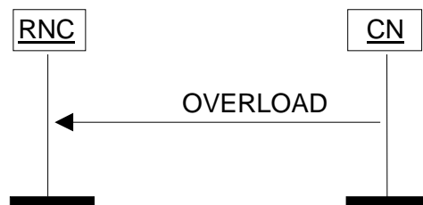
Figure 27: Overload at the CN. Successful operation.
