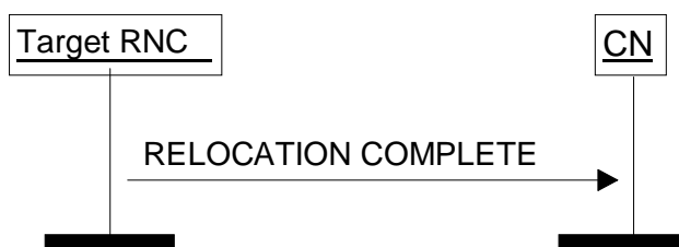
Figure 10: Relocation Complete procedure. Successful operation.
