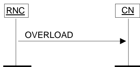
Figure 28: Overload at the UTRAN. Successful operation.
