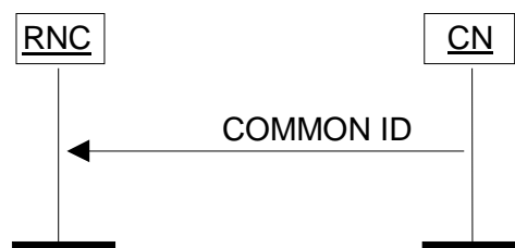
Figure 17: Common ID procedure. Successful operation.
