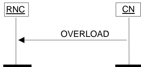
Figure 27: Overload at the CN. Successful operation.
