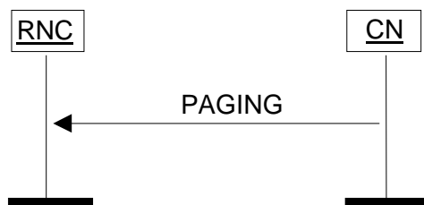
Figure 16: Paging procedure. Successful operation.
