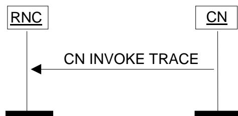
Figure 18: CN Invoke Trace procedure. Successful operation.
