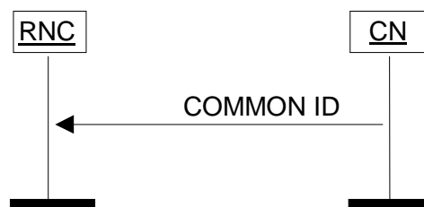
Figure 17: Common ID procedure. Successful operation.
