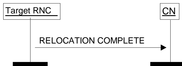
Figure 10: Relocation Complete procedure. Successful operation.
