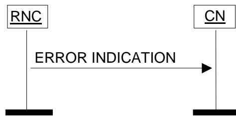
Figure 32: Error Indication procedure, RNC originated. Successful operation.
