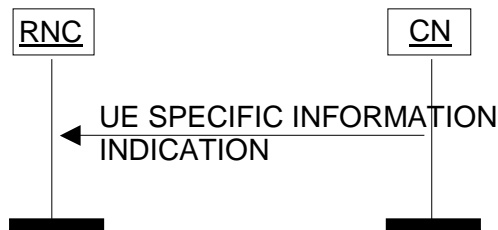
Figure 41: UE Specific Information procedure. Successful operation.
