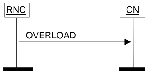
Figure 28: Overload at the UTRAN. Successful operation.
