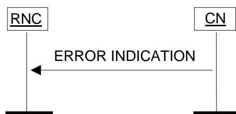
Figure 31: Error Indication procedure, CN originated. Successful operation.
