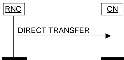
Figure 26: Direct Transfer, RNC originated. Successful operation.
