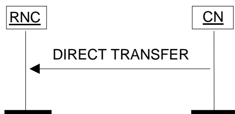
Figure 25: Direct Transfer, CN originated. Successful operation.
