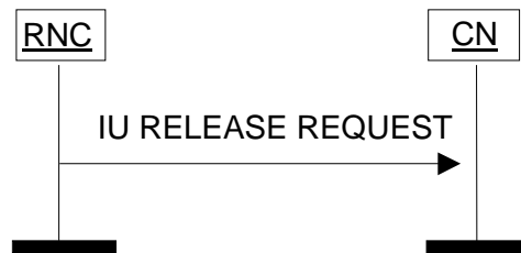
Figure 3: Iu Release Request procedure. Successful operation.
