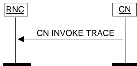
Figure 18: CN Invoke Trace procedure. Successful operation.
