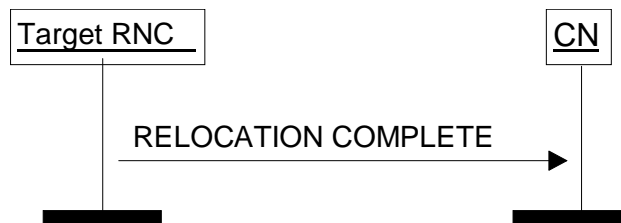
Figure 10: Relocation Complete procedure. Successful operation.
