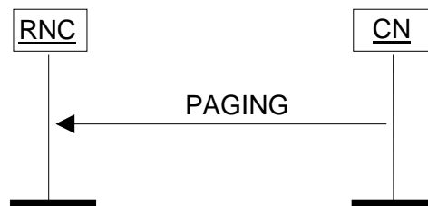
Figure 16: Paging procedure. Successful operation.
