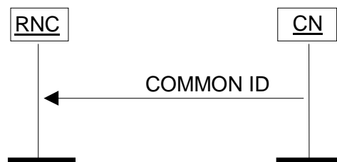
Figure 17: Common ID procedure. Successful operation.
