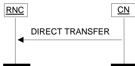
Figure 25: Direct Transfer, CN originated. Successful operation.
