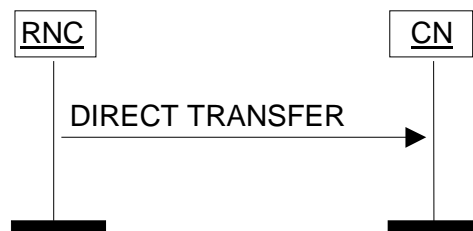
Figure 26: Direct Transfer, RNC originated. Successful operation.
