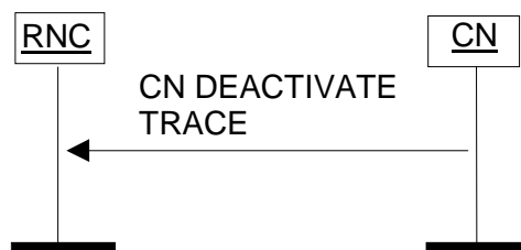
Figure 33: CN Deactivate Trace procedure. Successful operation.
