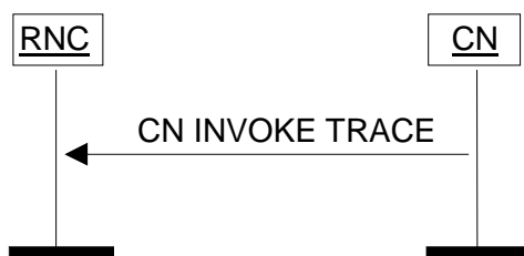
Figure 18: CN Invoke Trace procedure. Successful operation.
