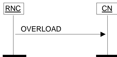
Figure 28: Overload at the UTRAN. Successful operation.
