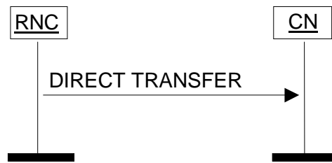
Figure 26: Direct Transfer, RNC originated. Successful operation.
