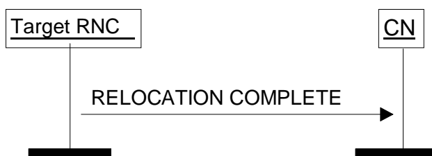
Figure 10: Relocation Complete procedure. Successful operation.
