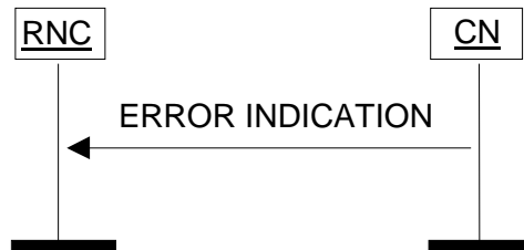
Figure 31: Error Indication procedure, CN originated. Successful operation.
