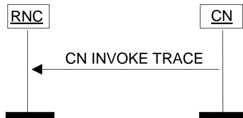
Figure 18: CN Invoke Trace procedure. Successful operation.
