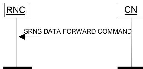
Figure 13: SRNS Data Forwarding Initiation procedure. Successful operation.
