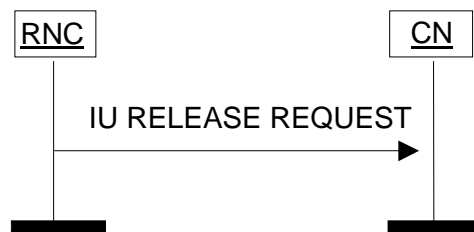
Figure 3: Iu Release Request procedure. Successful operation.
