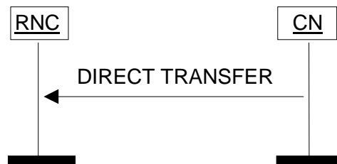
Figure 25: Direct Transfer, CN originated. Successful operation.
