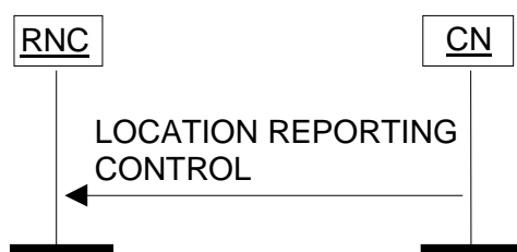
Figure 21: Location Reporting Control procedure. Successful operation.
