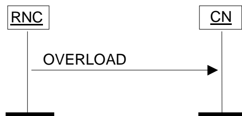
Figure 28: Overload at the UTRAN. Successful operation.
