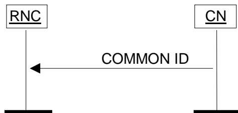
Figure 17: Common ID procedure. Successful operation.
