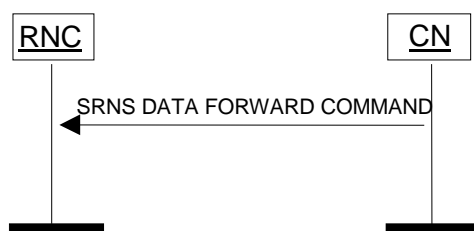
Figure 13: SRNS Data Forwarding Initiation procedure. Successful operation.
