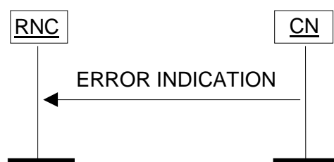
Figure 31: Error Indication procedure, CN originated. Successful operation.
