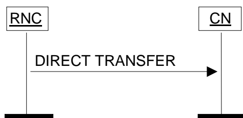
Figure 26: Direct Transfer, RNC originated. Successful operation.
