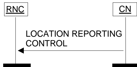
Figure 21: Location Reporting Control procedure. Successful operation.
