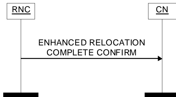
Figure 70: Enhanced Relocation Complete Confirm procedure. Successful operation.
