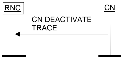
Figure 33: CN Deactivate Trace procedure. Successful operation.
