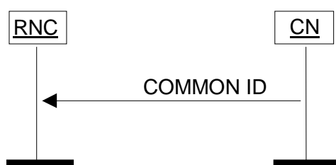
Figure 17: Common ID procedure. Successful operation.
