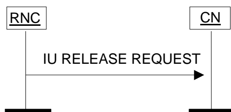
Figure 3: Iu Release Request procedure. Successful operation.
