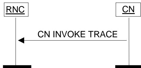
Figure 18: CN Invoke Trace procedure. Successful operation.
