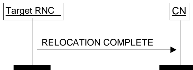
Figure 10: Relocation Complete procedure. Successful operation.
