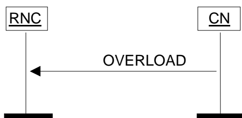
Figure 27: Overload at the CN. Successful operation.
