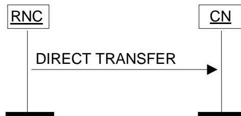
Figure 26: Direct Transfer, RNC originated. Successful operation.
