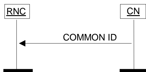
Figure 17: Common ID procedure. Successful operation.
