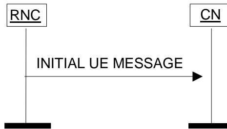
Figure 24: Initial UE Message procedure. Successful operation.
