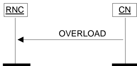
Figure 27: Overload at the CN. Successful operation.
