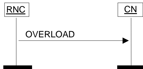
Figure 28: Overload at the UTRAN. Successful operation.
