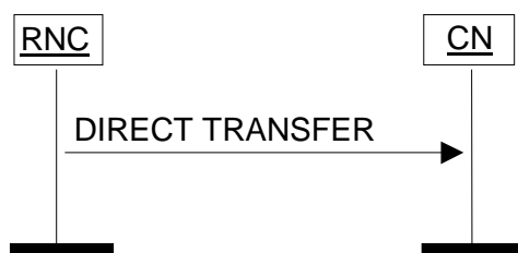
Figure 26: Direct Transfer, RNC originated. Successful operation.
