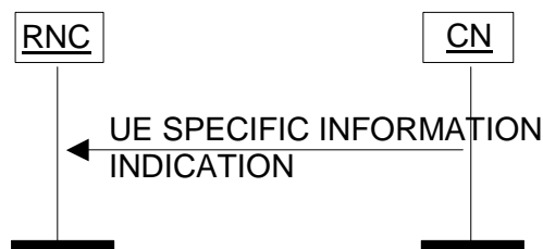
Figure 41: UE Specific Information procedure. Successful operation.
