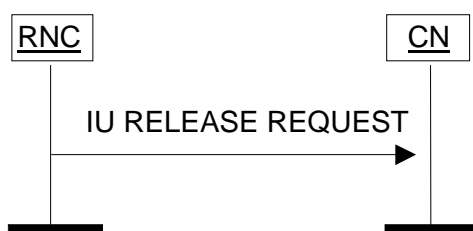
Figure 3: Iu Release Request procedure. Successful operation.
