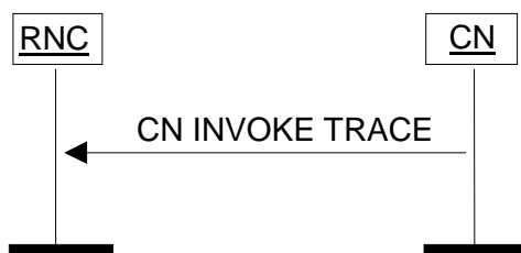
Figure 18: CN Invoke Trace procedure. Successful operation.
