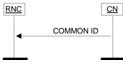
Figure 17: Common ID procedure. Successful operation.
