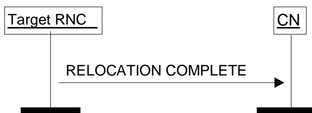
Figure 10: Relocation Complete procedure. Successful operation.
