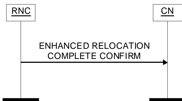
Figure 60: Enhanced Relocation Complete Confirm procedure. Successful operation.
