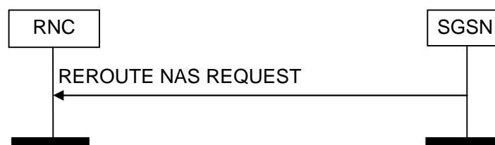
Figure 64: Reroute NAS Request procedure: Successful operation.
