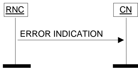
Figure 32: Error Indication procedure, RNC originated. Successful operation.
