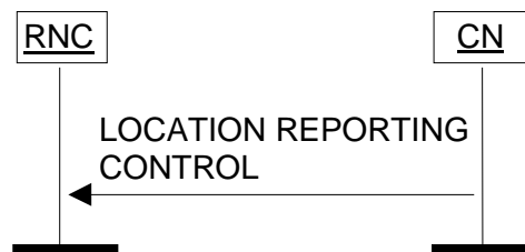
Figure 21: Location Reporting Control procedure. Successful operation.
