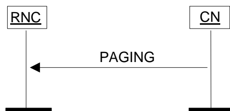
Figure 16: Paging procedure. Successful operation.
