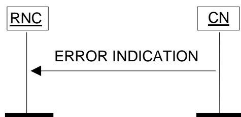
Figure 31: Error Indication procedure, CN originated. Successful operation.
