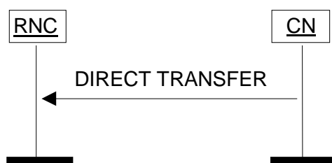
Figure 25: Direct Transfer, CN originated. Successful operation.
