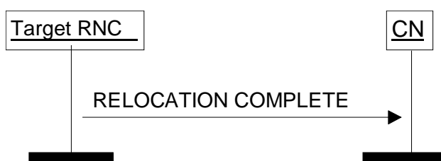
Figure 10: Relocation Complete procedure. Successful operation.
