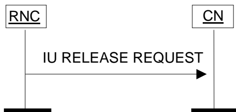
Figure 3: Iu Release Request procedure. Successful operation.
