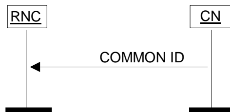
Figure 17: Common ID procedure. Successful operation.
