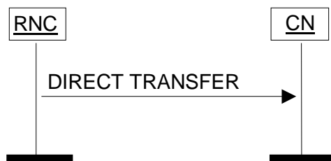
Figure 26: Direct Transfer, RNC originated. Successful operation.
