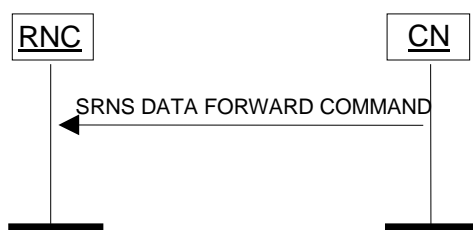
Figure 13: SRNS Data Forwarding Initiation procedure. Successful operation.
