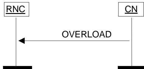
Figure 27: Overload at the CN. Successful operation.
