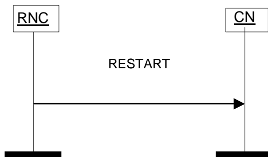
Figure 11: Restart Indication Procedure: Successful Operation
