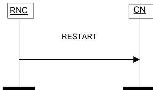
Figure 11: Restart Indication Procedure: Successful Operation
