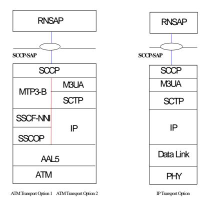
Figure 1: Signalling bearer for RNSAP
