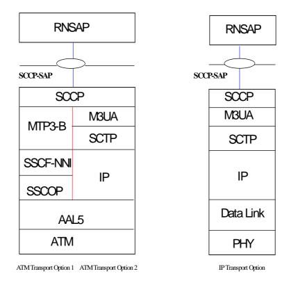
Figure 1: Signalling bearer for RNSAP
