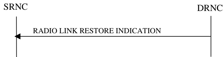
Figure 19: RL Restoration procedure, Successful Operation
