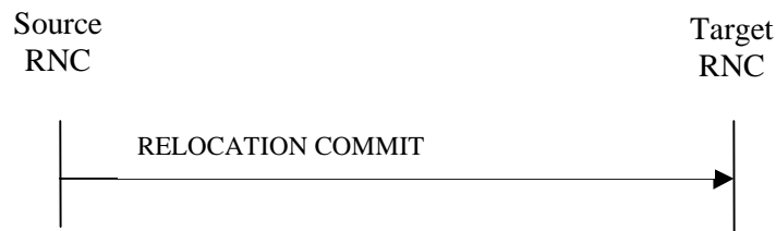
Figure 3: Relocation Commit procedure, Successful Operation
