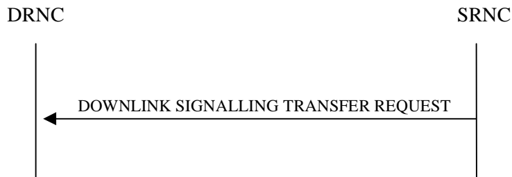
Figure 2: Downlink Signalling Transfer procedure, Successful Operation
