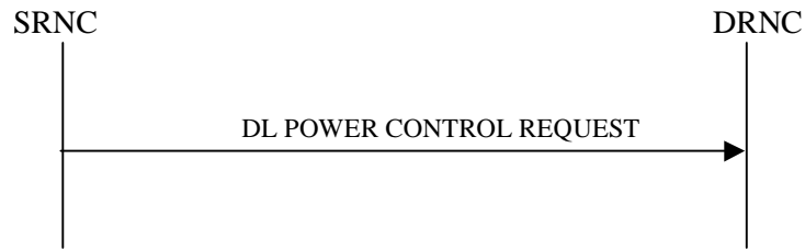
Figure 25: Downlink Power Control procedure, Successful Operation
