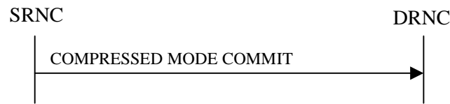
Figure 28: Compressed Mode Commit procedure, Successful Operation
