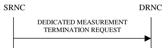
Figure 23: Measurement Termination procedure, Successful Operation
