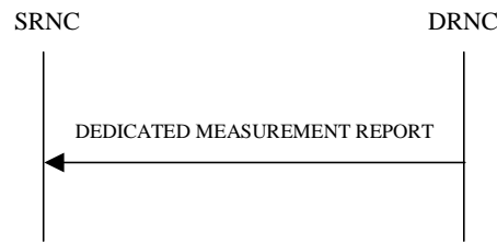
Figure 22: Measurement Reporting procedure, Successful Operation
