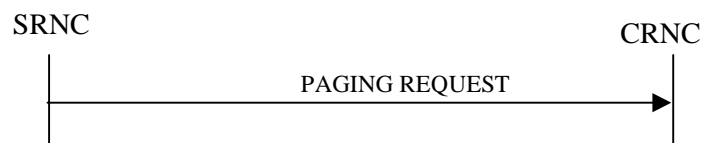
Figure 4: Paging procedure, Successful Operation
