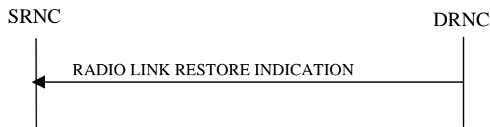
Figure 19: RL Restoration procedure, Successful Operation
