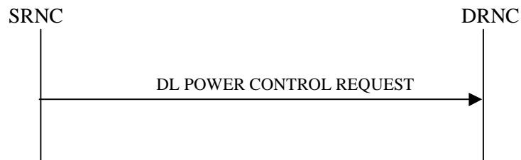
Figure 25: Downlink Power Control procedure, Successful Operation
