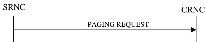
Figure 4: Paging procedure, Successful Operation
